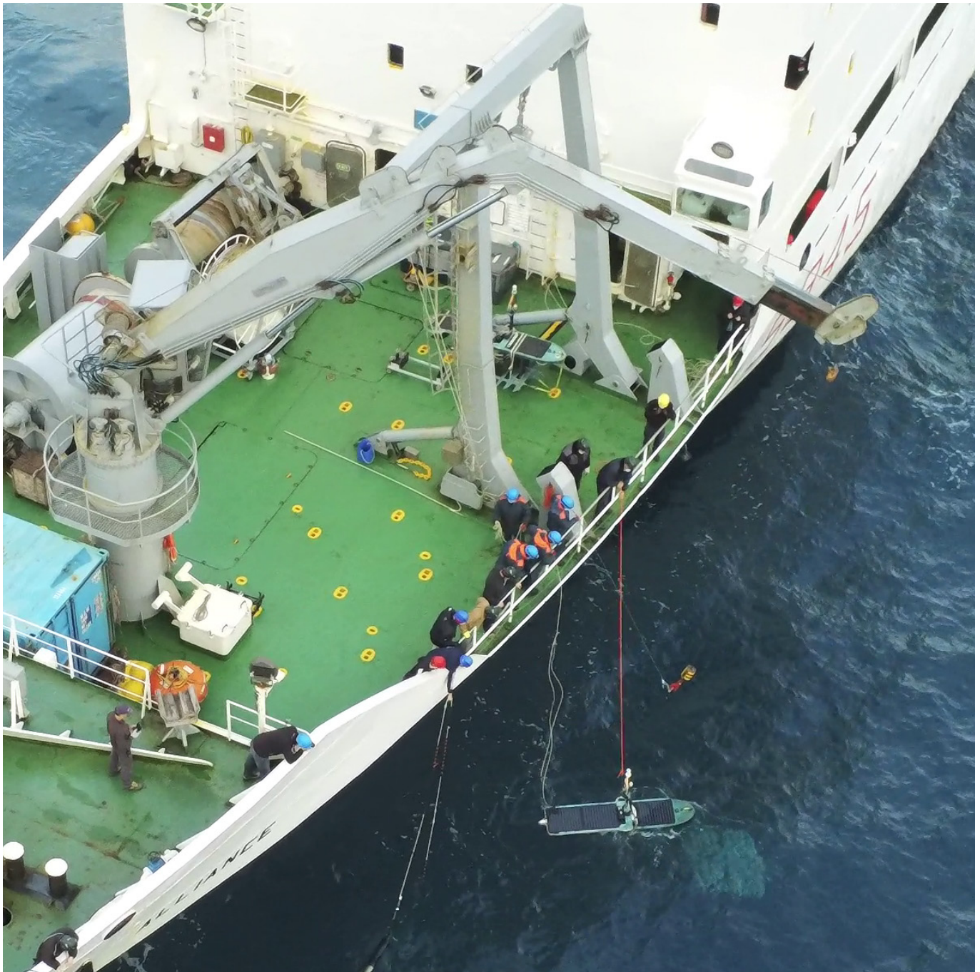
A wave glider, part of the underwater communications network, is deployed from NRV Alliance during the Distributed Autonomous Networked Systems sea trial in December 2020.
