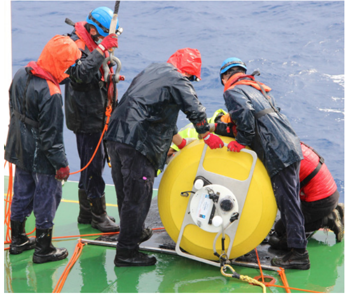
CMRE researchers and ITA N crew members deploy a Wirewalker in the rain from NRV Alliance during the MREP20 sea trial in the Strait of Sicily.
