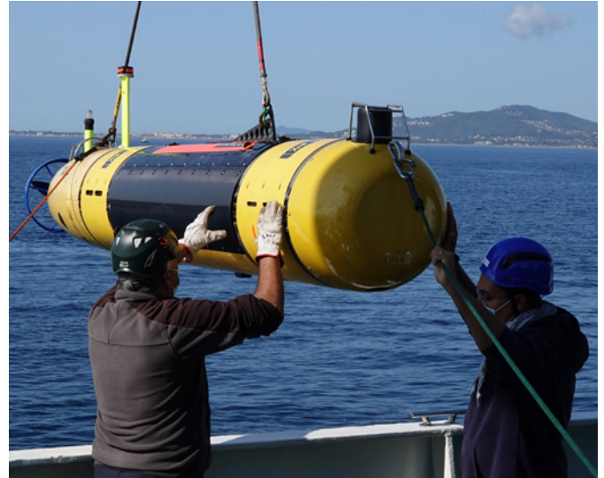
The CMRE team deploy the MUSCLE AUV from NRV Alliance during DYNAMIC MARINER 2020.
