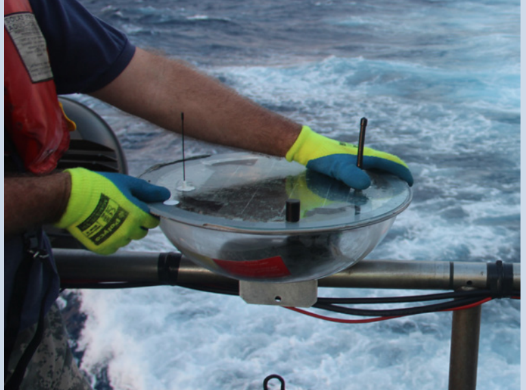
A CMRE technician prepares to deploy an autonomous drifter to characterize the maritime environment off Italy.
